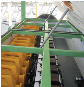
Home Battery Kits recharging from the STAR trailer
